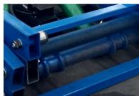
Axle pin:45 # round steel, quenching and tempering.
