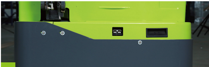
Charging interface, external intelligent charger, convenient and safe
