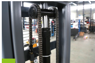
Thick hydraulic cylinder, double chain
