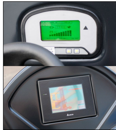
Camera and positioning: Optional positioning system offers easier pallet handling at height through camera system.
