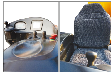
Suspension seat is adjustable; light steering wheel with armrest.
